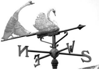
design in front of the pivot point has a smaller surface area than the part behind it. The wind exerts more force on the larger end, moving the vane around so that the smaller end faces the direction from which the wind is blowing. The main points of the compass are indicated below, so that knowledgeable observers may be able to predict what type of weather will ensue.
